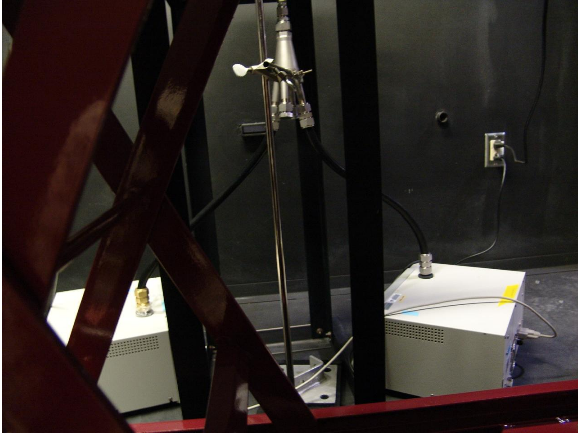
Figure 12: Tubing connecting two branches of one-to-four flow splitter to two aerodynamic particle sizers
