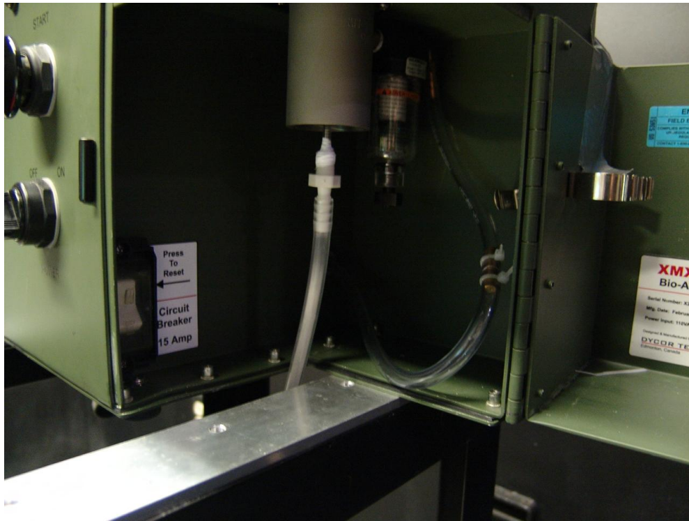
Figure 9: Special connector and tubing connected to liquid impinger tube
