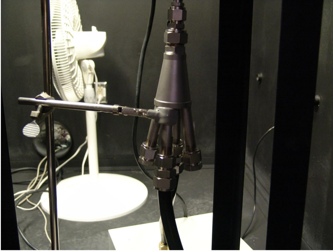
Figure 13: Two branches of one-to-four flow splitter capped
